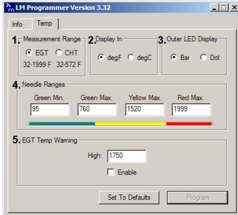
1. **Measurement Range:** In *EGT* range the gauge will display the temperature with a X 10 multiplier to allow for 4 digit numbers. In *CHT* range the gauge will display the three digit temperature (no multiplier).
