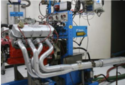
**2** After testing with lab gas the sensors were run-in for an hour with race fuel, on a test engine (Westech just happened to have a Chevy motor in the dyno room that day.) The run in simulates the wear and tear a sensor goes through with live fuel and heat conditions.
