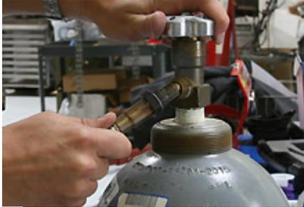
**1** Sensors were tested using laboratory gas specifically formulated to yield 11.76 AFR and 13.15 AFR. This way each sensor sees the exact same "exhaust gas", letting us measure the accuracy and responsiveness of each meter.
